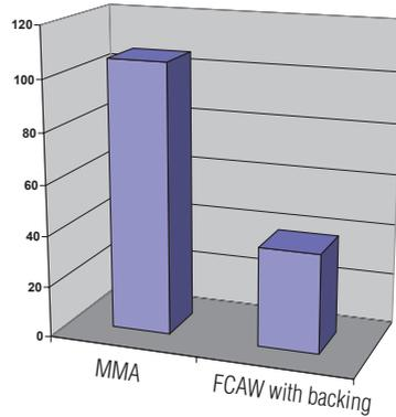
Typical deposition rate is 2,5-3,0 kg/h.
